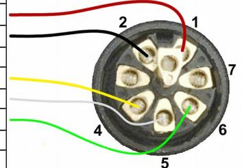
Fig. 2: Female connector back view with connection scheme
